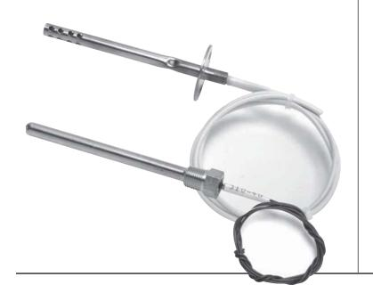
The 310 Thermistor Sensors must be wired in series with a 320 Setpoint Adjuster or 205 Step Control . The total resistance is 2200 ohms when the setpoint equals the sensor temperature. The NTC thermistor increases resistance as temperature decreases.
